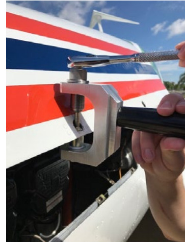
For portable field repair, use Skybolt® tool dies with the Skybolt® SK-2018 Clamp as shown here installing new ZLoc® studs/grommets on a Beech Bonanza.
