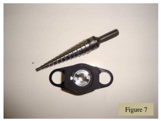
Drill mount holes to 7/16" with Unibit-1 drill
