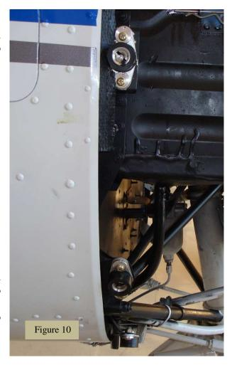
Step 20 – (1/2 Hour) Position Lower Cowling as described in Step 17. Position the Upper Cowling. Install one or two SK40S5S fasteners in Upper Cowl firewall holes and lock. (Note: If studs appear to be tight or not lock, do not force to lock. A longer stud is required).
