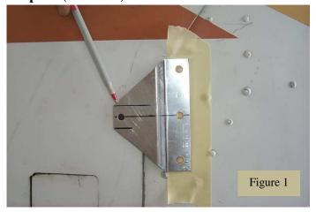
Place 8" strips of 1" masking tape behind the rivet line on the boot cowl adjacent to each stud as noted in picture. Sight template over each stud and mark holes onto tape. This important step will greatly enhance the alignment of each SK2003 mount at each location.
