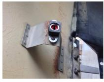
When Cessna developed the cowling mount system for the C150, C172, C177, and some C182 airframes, they apparently took into consideration that the mounts could fail and the cowling could come in contact with the prop spinner. On some models, they installed a snubber (the same J7444 mount used around the firewall) at the nose of the
