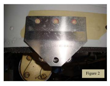
This is all too common on many Cessna cowling mounts. Without the SK203-TEM1, it would be difficult to tell just how much each mount is off from its respective cowling hole. To move a mount far enough to center (as in this case), this mount will need to be modified for SK2003-AW4 Camwashers.
