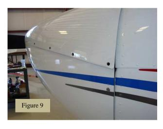
With Lower Cowl fastened, and Upper Cowl in position, stripes are in line, side edge is properly positioned with paint line, and side holes are in line.
