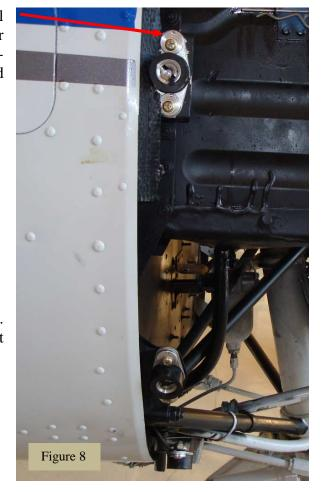
**Step 19** – (1 **Hour**) **Re-install modified SK2003-42 Mounts**. "Dial" the Camwashers to the desired offset to achieve alignment goals.
