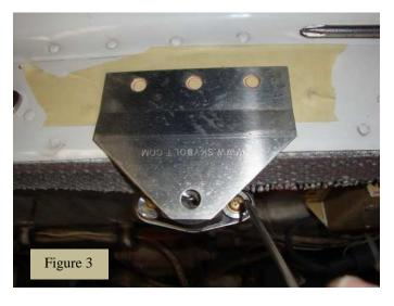
Step 2 - Remove Upper Cowling (Leave Lower Cowling on Aircraft). If you are *not* converting the side fasteners, place a piece of tape over the rear hole of the side cowling to prevent drilling in Step 5.
