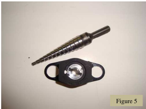
Drill mount holes to 7/16” with Unibit-1 drill
