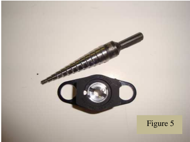
Drill mount holes to 7/16” with Unibit-1 drill
