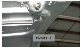
The existing Dzus® Fastener is removed by lifting the aluminum grommet so the grommet and stud may be removed from the cowling. Use long-billed, angled pliers or nail cutter to work the grommet from the backside.
