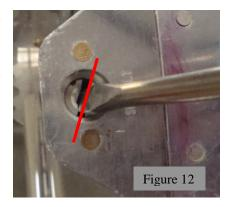
9) Reinstall the panel and lock all fasteners. Check for proper locking torque and proper alignment. Adjust the receptacle insert for proper depth by inserting a thin pick to raise the locking collar. See Figure 13 on page 9.
