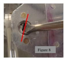
9) Close cowling and lock all fasteners. Check for proper locking torque and proper alignment. Adjust any receptacle for alignment and adjust the receptacle insert for proper depth by inserting a thin pick to raise the locking collar.
