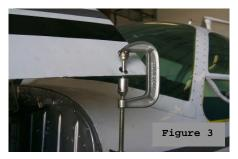
To install the new *ZLoc*® Fastener in the Bonanza cowling, the Skybolt SK-A5 or SK-A5C tool is required. Follow the instructions supplied with the tool set to seat the grommet and fastener assembly. Note: Standard Dzus® tooling will not install the assembly without removing the support bracket from the airframe.
