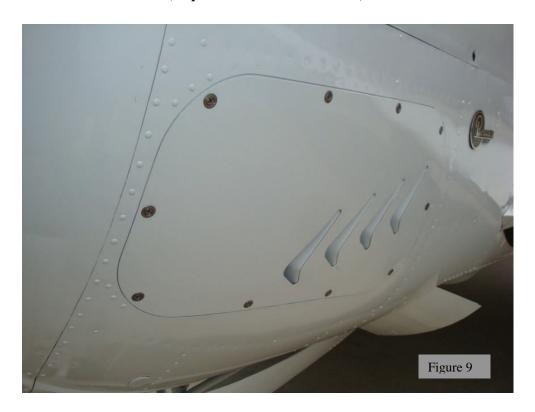
Like the upper cowling, replacement of fastener receptacles is simple because of the exact same rivet size and spacing (.750"). If the receptacles used on your aircraft have 1.000" rivet spacing, this kit will not work. Use B35LC40 Kits for the larger fasteners.
