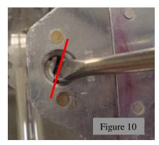
8) Reinstall the panel and lock all fasteners. Check for proper locking torque and proper alignment. Adjust the receptacle insert for proper depth by inserting a thin pick to raise the locking collar. See Figure 13 on page 9.
