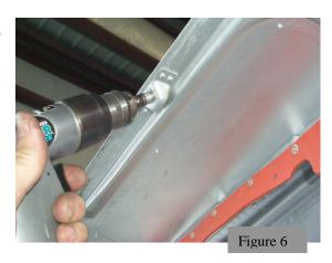
6) Install the SK-OS grommet and R4G retainer with T26 Tool.
