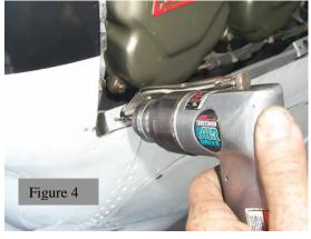
2) Drill out and remove old locking springs from mounting brackets. Clamp the spring or simply loop a TyWrap around the spring to prevent it from falling.
