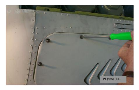
First, insure that your aircraft used the large #5 Airlocs® in the Gill Panel. The simplest way to tell is to measure the rivet spacing on the receptacle. This should be 1.000". If it is .750", this kit will not work. (Use kit B35LC2700/2800 Series Kits if #2 Airlocs are on your aircraft - .750" rivet spacing)
