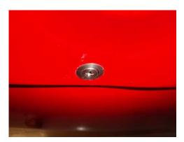
8) Re-install the stud. Lock and note that it is correctly adjusted as to not be too tight (requiring force to lock) and is flush with the face of the grommet. Many times, particularly for engine cowlings that typically have mis-faced surfaces, or in the case of Cessna firewall platemounts, there is a large adjustment between just flush and a properly set tension for positive lock without being too tight.
