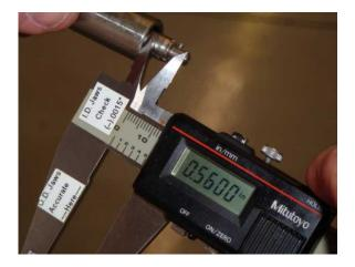
5) Remove the tool and measure the distance from the end to the sleeve, in this case it is .560.
