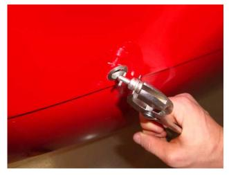
4) Loosen the adjuster sleeve set screw and insert the tool into the receptacle as far as it will allow. Slide the adjuster sleeve until it faces with the grommet and tighten the set screw.
