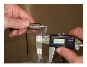
6) Reset the adjuster sleeve to .560 plus .100 = .660 as shown and tighten the set screw. This should establish a target depth for all panel fasteners assuming a uniform panel thickness.
