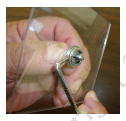
Over the years we have been working on, building, or converting cowling fasteners, one of the most annoying parts of the job is removing old grommet retainers for the Camloc 4000 Series. For years, we have recommended using a curved pick tool and cleverly "picking" the snap ring retainer off of the back side of the grommet.
